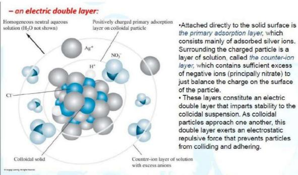
Figure 12.1 A colloidal silver chloride (AgCI) suspended in a solution of excess AgNO<sub>3</sub>
