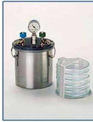
( Anaerobic Jar )
